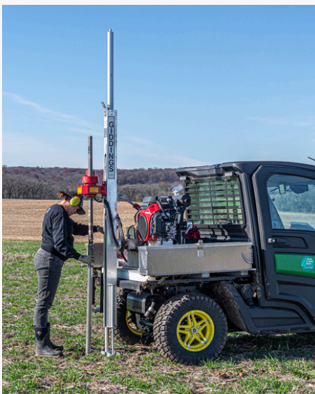
Staff utilize a soil probe mounted to a UTV to collect samples to a depth of one meter.
